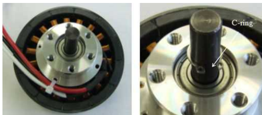
Fig. 9. Assemble the rotor unit and set the c-ring
