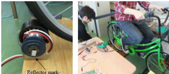
(c) Generator driven by rear wheel (d) Experiment by bicycle drive
