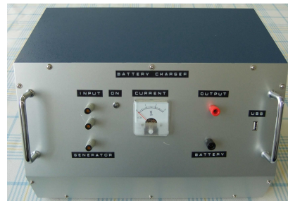
Fig. 20. Constant current-constant voltage charger
