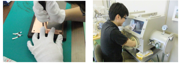
(a) Spot welding (b) Vacuum glove box Fig. 24. Spot welding of electrode terminals and operation inside the vacuum glove box
