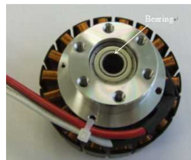
Fig. 8. Set the bearing to the stator base hole
