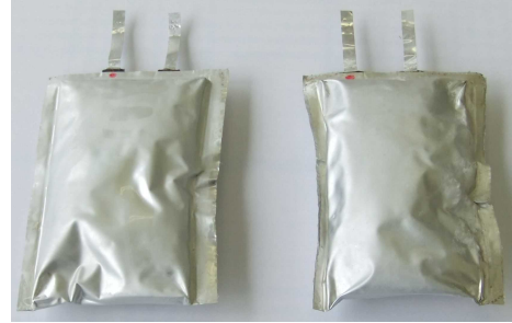
Fig. 25. Laminate type lithium ion battery
