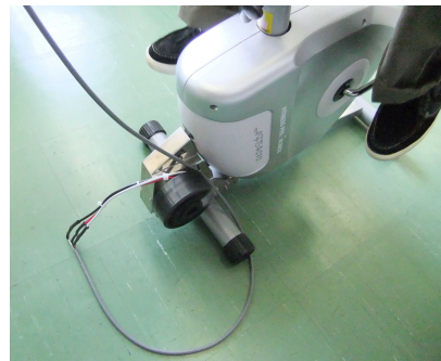
Fig. 19. Generator mounted to an exercise bike
