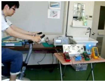
Fig. 22. Charging experiment by an exercise bike
