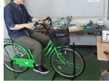
(a) Pedaling a bicycle with two dynamos mounted
