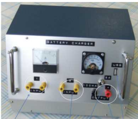
Fig. 9. Lithium ion battery charger using two dynamos
