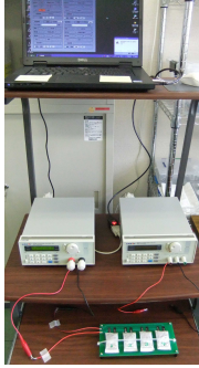
Fig. 13. Charging and discharging evaluation device for lithium ion battery
