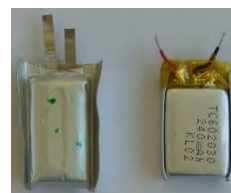
Fig.5 Li-Ion(left) manufactured by us and Li-Po battery(right)
