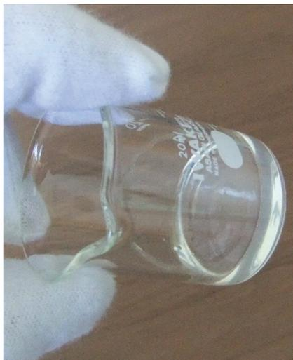
**Figure 1:** Gelation of electrolyte solution (1 mol LiTFSI in PC)
