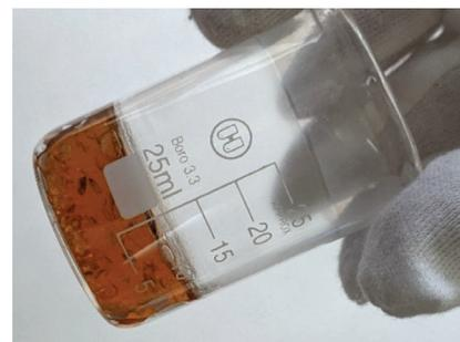
**Figure 2:** Gelation of electrolyte 1 mol LiPF<sub>6</sub> in EC/DEC (1:1 vol%)
