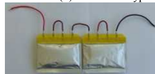
(c)Li-Ion battery stack
